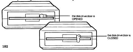
Before you can use a disk, it must be *initialised*. You do this with the command INIT. When you type this in, and press RETURN, you'll see the red light on the disk drive come on. Never try to remove a disk while the red light is on. After some whirring noises, which will continue for quite a while, the light will go out, and the disk will be initialised. Note that the initialisation process wipes *everything* on a disk, so make sure you use this command with care.
