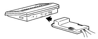
The controller communicates with the disk drive or drives via a 20-pin connector which provides all input/output signals.
