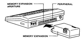
To check that the extra memory is correctly inserted, you type in PRINT PEEK (30897) and press the RETURN key, which should give you an answer of 255. Then, if you tyupe in PRINT PEEK (30898) and press RETURN, you'll get 247.
